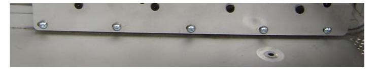
tray with 4 more of the screws (again please note the screw type now used are SILVER with a CROSS HEAD type and <u>not</u> the black screws with allen head shown) and then use the 5 longer silver screws with allen/hex head and washers to join the "bridge" to the case screw mount points.
