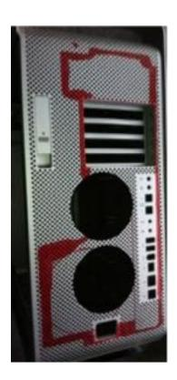
After you have stripped the G5 completely, start by masking the area where you will be cutting and using a rotary tool (e.g. Dremel) make your cuts.
