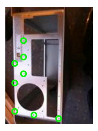
Then attach the IO shield using screws, nuts and washers for the orange circled positions and just screws for the yellow positions. Note that for the long side of the IO plate the yellow holes on the shield are already tapped. Don't do these screws up too tightly as the threads at that point can be stripped if they are overtightened.
