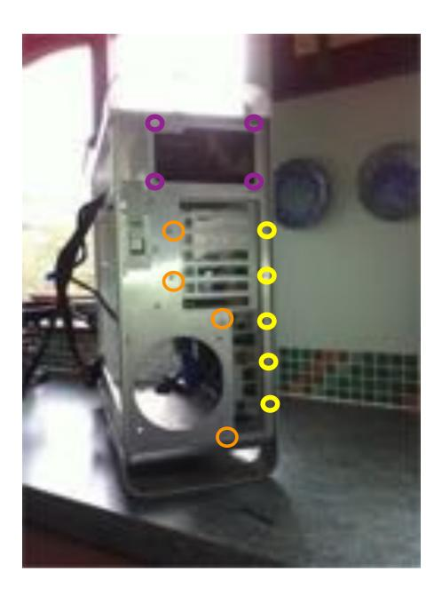
Then test fit your ATX supply (screws shown in purple). Note that any obstructions to fitting the PSU need to have been removed before this - notably the shelf must be removed.
