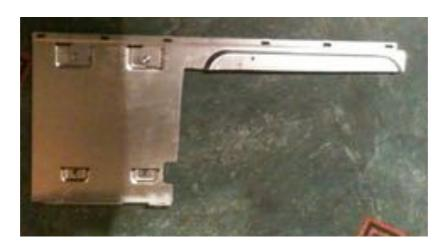
Dependent on your build, you may wish to cut either more or less of the shelf than shown and use it to help support the weight of the power supply. In our experience so far at the Laser Hive, we have not found it necessary to use the shelf to provide any extra support to the PSU enclosure. However, if you have a particularly long/ heavy power supply you might wish to provide extra support by using, for instance, a simple piece of right angle bracket attached to the shelf extra weight support.
