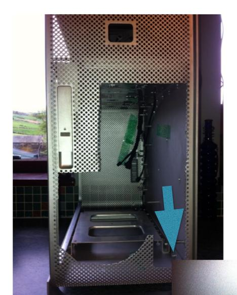
The four rear most of the lower case screws mounting points- i.e. referring to the photo to the right, the blue arrow indicates one of the case screw mounts.
