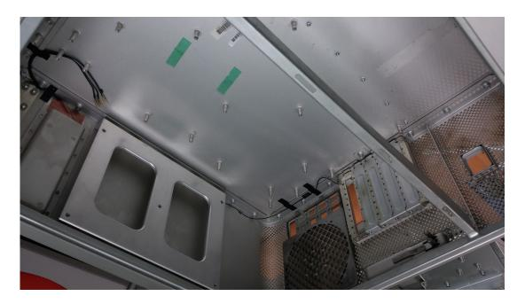
If your Mac Pro has an internally fastened lower shelf as shown in the photo above (i.e. a shelf at the bottom of the case with a support as shown) then this lower shelf support must be removed. This will need to be painstakingly cut out before the concealed fixings can be reached
