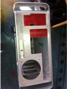
Start by masking the area where you will be cutting and using a rotary tool (e.g. Dremel) cut out the original IO section.
