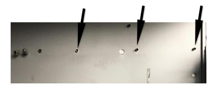
Next remove the three rear most case screws to expose the mounts at the bottom rear of the case as shown below. ( Note: Mac Pro uses 3 instead of 5 bottom case screw mounts).
